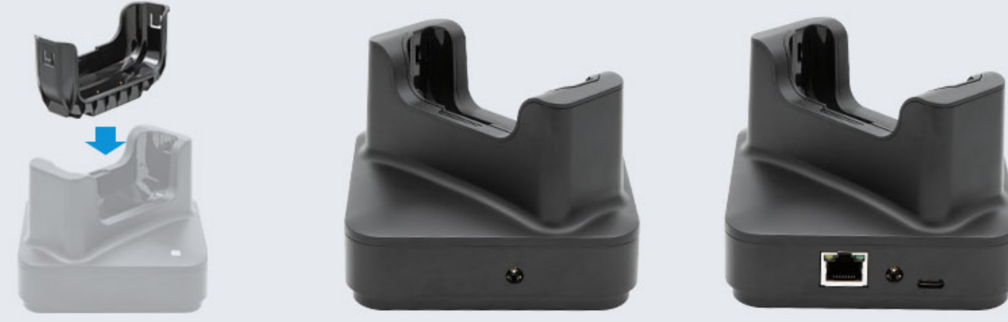
CRD-C72-RBC/CRD-C72-RBCE Charging Cradle for device, use with DCPWR-12V2A-XX adaptor. CRD-C72-RBCE is an advanced CRD-C72-RBC, w/sync, w/ethernet, w/DC. The cradle cup has an insert that must be removed prior to inserting the C72 with Rugged Boot.
